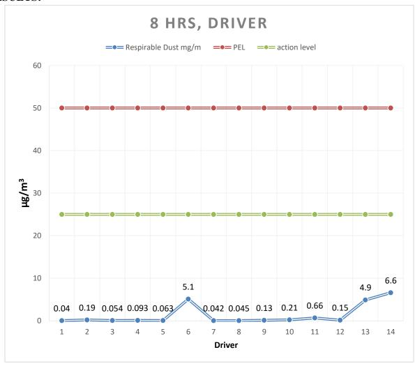
**CONCLUSION:** All samples were below the OSHA PEL for respirable dust and silica species. Testing conducted under normal working conditions. Data assessment subject to change outside the scope of normal working conditions.
