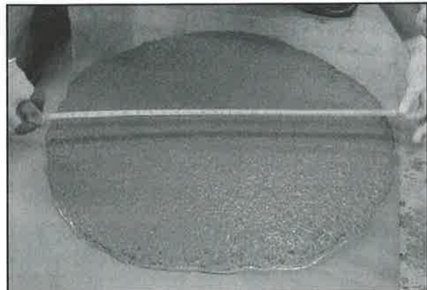
Figure 1: SCC with a slump flow of 29-inches (725-mm) tested by the slump flow test
